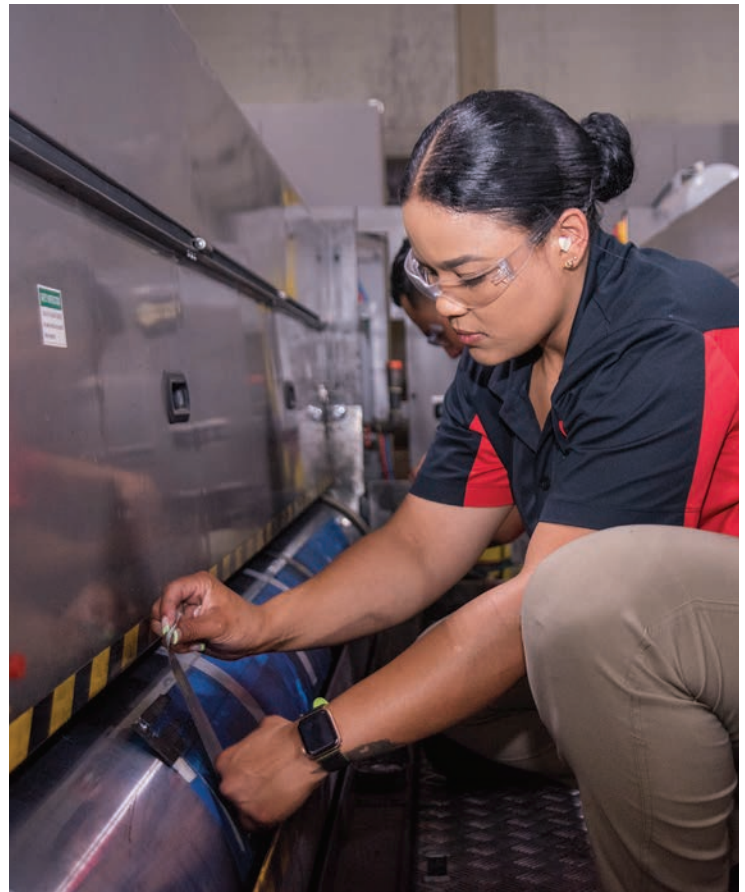
Utility Coordinator Estefani Gil pre-setting a print plate for the next job at the EVOL 115 machine center.
