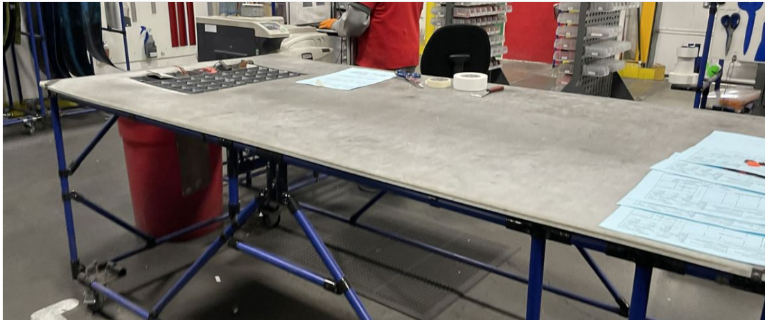
A hole has been made in the HDPE of this modular table to facilitate the accessibility of small frequently used parts.
