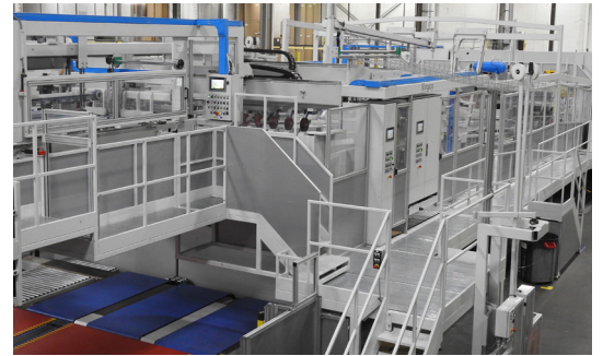
President Container Group's new Engico dual-sized 66/99-inch Jumbo Flexo Folder Gluer.
